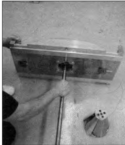
Step 2 First, attach the impeller shaft to the motor spindle.
