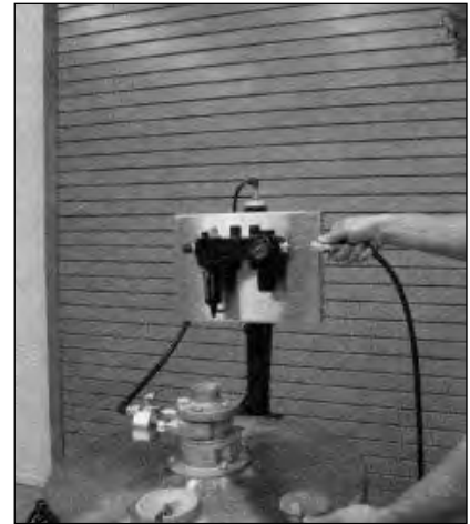
Step 3 With the JBW Mixing Lift System secured, attach a 1/4" or larger air line to the inlet air regulator.
