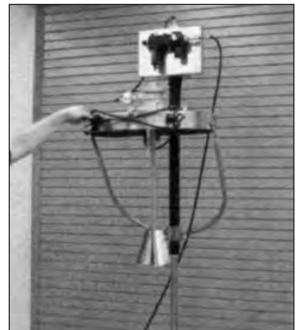
Step 6 To allow for proper placement of the drum, the JBW Mixing Lift System should be in the full up position. To reach the full height, hold the LEFT up-down safety switch until the unit stops.
