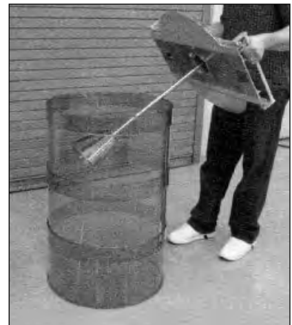
Step 6 To place the portable drum mixer or tote® mixer into the drum, first grasp the handles and guide the impeller and shaft gently into the drum opening.
