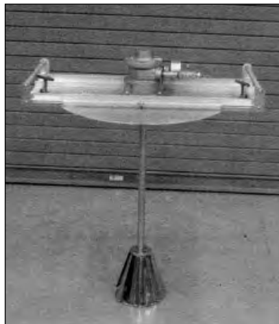
Step 5 The portable drum or tote® mixer can be easily transported to the drum/ tote® tank rather than the drum being moved to a stationary mixing system.
