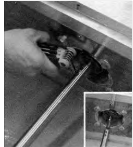
Step 3 Using a hex head wrench, secure impeller shaft to the motor spindle. Note: When securing the shaft to the motor spindle, align the hex head screws with the key way. This will eliminate the possibility of the motor spindle slipping when mixing higher viscous fluids.
