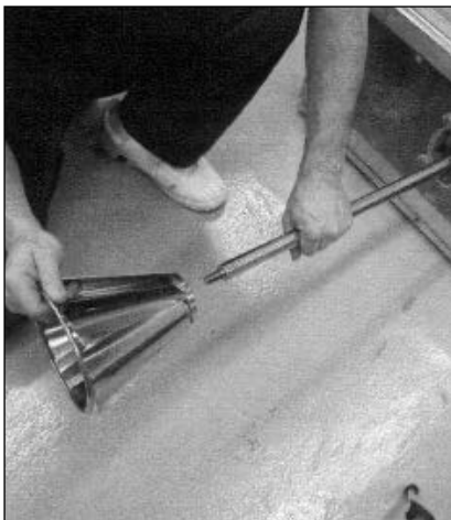
Step 4 Install the impeller by threading the impeller onto the shaft with the large end facing down as shown in the picture.
