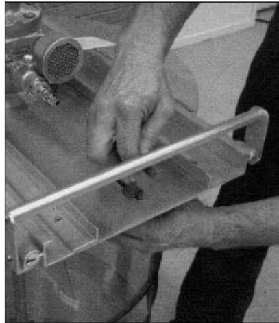
Step 8 After the drum or tote® mixer is positioned in the drum, secure the mixer to the drum using the drum clamp assembly.
