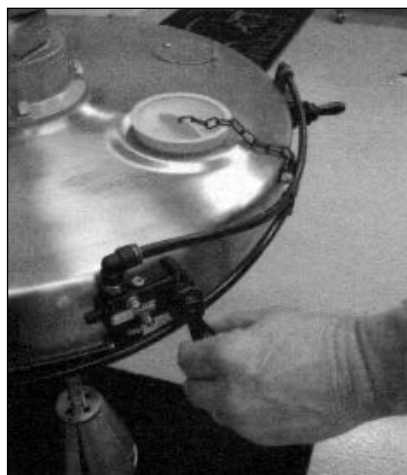
Step 5 After adjusting the inlet air regulator, move the JBW Mixing Lift System in the up position by maneuvering the LEFT up-down safety switch.
